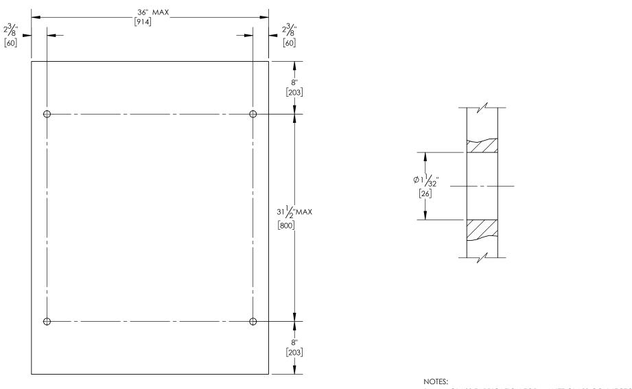
1. GLASS FABRICATION FOR MANET GLASS CONNECTOR FOR 3/8" AND 1/2" MONOLITHIC GLASS
